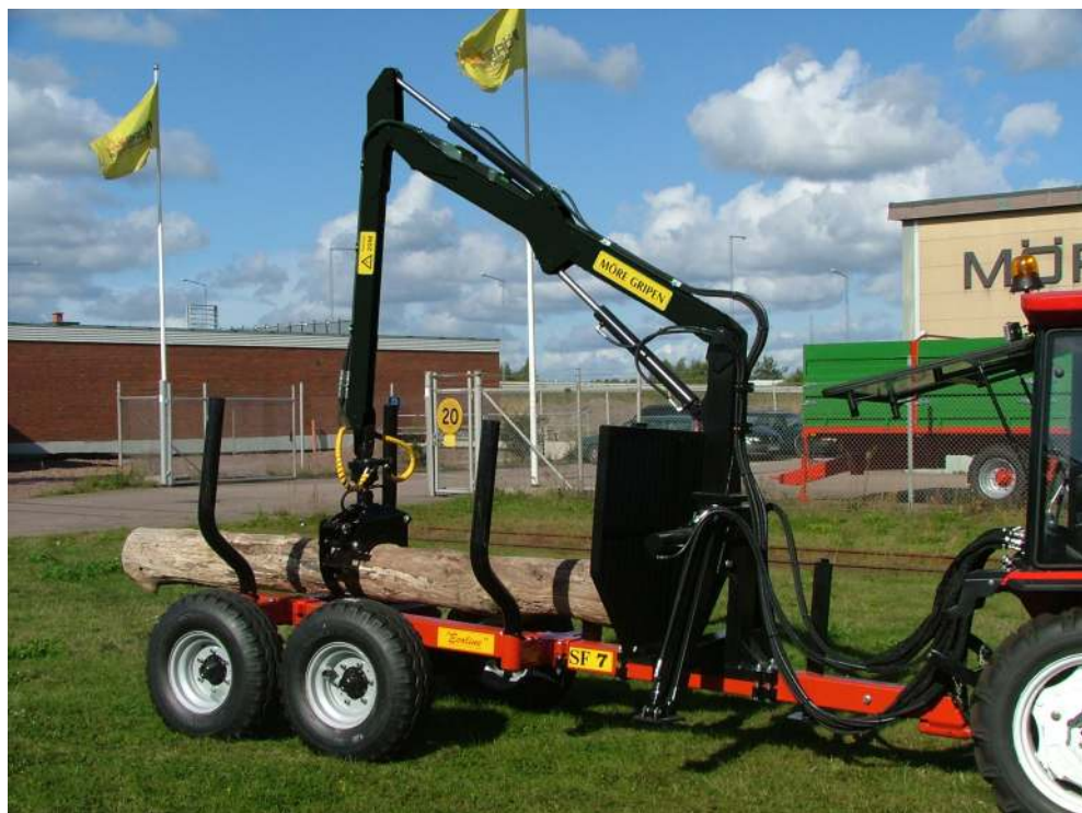
Forestry trailer 7 tonnes, centre frame, bogie wheels, hydraulic support legs, pivoted supports, tow ring for tractor
